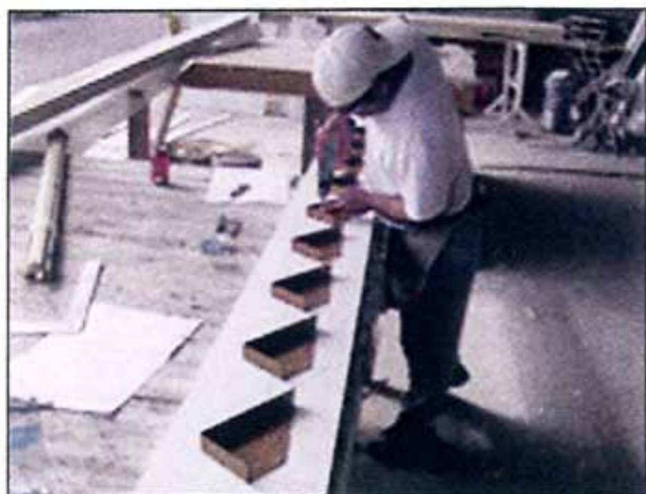
Left: A stair stringer is assembled using EZ Stairs' brackets in the Palm Harbor Homes factory. The brackets are screw attached and then swiveled into place, making stringer set up fast and easy for both risers and treads. This system provides for stair construction either in the plant (center photo) or at the home site. At right a Palm Harbor model featuring stairs built with the EZ Stairs system.
